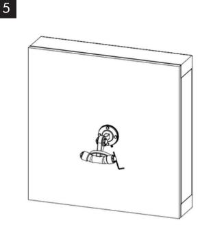
Place the robe hook onto the mount. Using the provided hex key, tighten the set screws down to secure the robe hook to the mounting tab.
