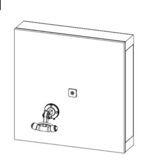
(DRYWALL): Using the provided 1/4-20 machined screw, secure the mounting tab to the finish wall with the groove facing down.
