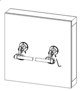
Using the provided hex key, tighten the set screws down to secure the robe hook to the mounting tab.
