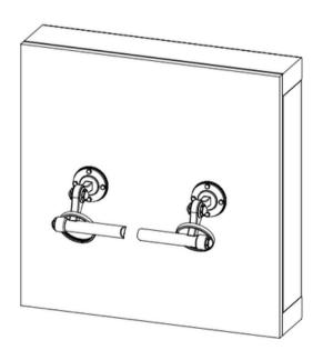
Carefully install both escutcheon rings onto the towel bar bases.
