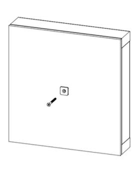
Using a 1/8" bit, predrill a hole in the previously marked location.
