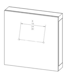
Determine desired install location. Mark locations of center to center. (Center to center will be dependent upon the towel bar length. 8", 18", 24" or 30".)
