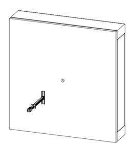
(Stud): If mounting to a stud, use the provided wood screw and fasten the mounting tab to the wall. (Ensure the mounting tab is level with the groove facing down.)
