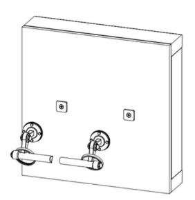
Place the towel bar onto the mounting tabs.
