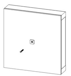
(Drywall): If there is no stud to mount to, drill a  $\frac{1}{2}$ " hole to push the supplied toggle through. Once the toggle is through the wall, slide the cap down the straps until it is flush with the finish wall. Snap off the excess from the straps.
