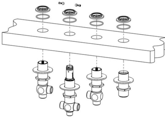
Disassemble top nut and o'ring seal from the top of the valves and cradle mount.
