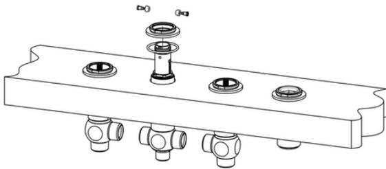
Place the diverter valve through the deck from underneath. Ensure one of the divot holes is facing toward the direction of the tub.
