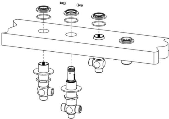
Place the cold (blue) valve through deck from underneath.
