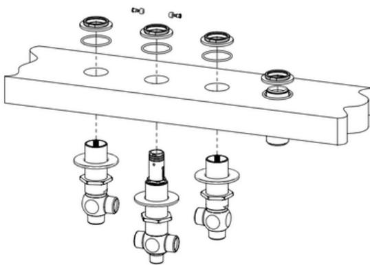
Tighten the top nut, with the o'ring seal in place, to the top of the handshower cradle until the top nut is flush to the top nut.
