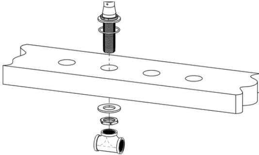
Place the spout anchor mount through the deck from the top of the deck.
