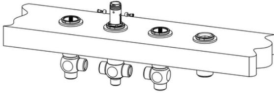
Secure in place from the bottom mounting nut.
