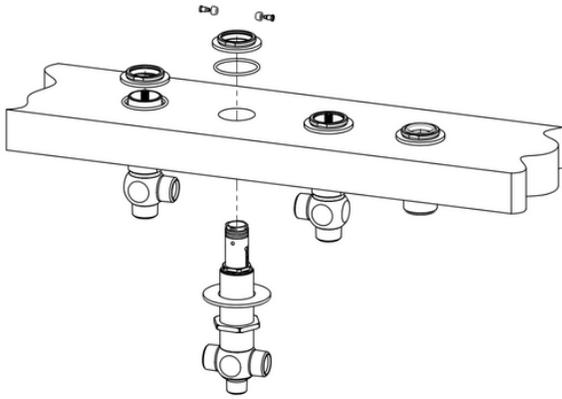
Tighten the top nut, with the o'ring seal in place, to the top of the hot valve until the top nut is bottomed out to the top of the valve.
