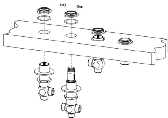
Tighten the top nut, with the o'ring seal in place, to the top of the cold valve until the top nut is bottomed out to the top of the valve.
