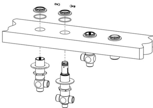
Secure in place from the bottom mounting nut.
