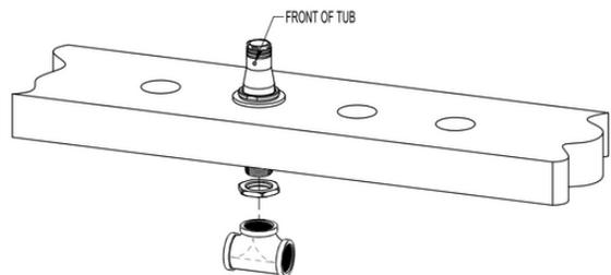
Ensure one of the divot holes is facing toward the direction of the tub.
