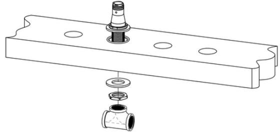
Secure the washer and mounting nut from underneath the deck.
