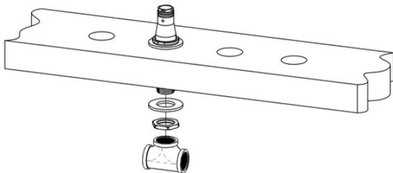
Apply plumbers' tape onto the bottom shank of the spout anchor. Secure the supplied tee connection to the bottom mount shank.
