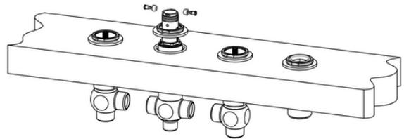
Tighten the top nut, with the o'ring seal in place, to the top of the diverter valve until the top nut is flush to the top of the valve.
