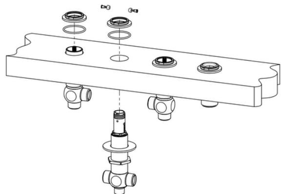
Place the hot (red) valve through the deck from underneath.
