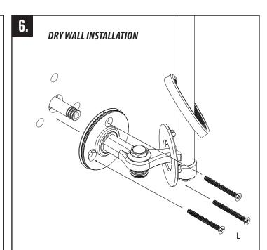
Apply non-petroleum based lubricant on the O-rings of the injector. Slide bottom bracket over the injector, ensure that it is level. Using the provided machine screws (L), secure both the dry and wet brackets to the finish wall using the toggle anchors.
