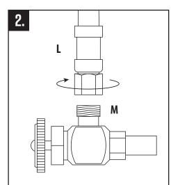
Before connecting supply hoses, flush supply stops to clear any debris. Place a bucket underneath stops and run water for 5 to 10 seconds. Turn water off. Carefully position hot and cold supplies so they will not interfere with other hoses. Connect supply hoses (L) to supply stops (M). Tighten nut by hand plus 1/4 turn with a wrench until snug. **DO NOT** use teflon tape or plumbers putty. Turn water back on and check for leaks.
