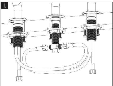
Carefully position all supply hoses so they will not interfere with each other. The inlet mix hoses are in front and do not have the hot or cold label. To avoid kinking, attach the inlet hoses to the opposite side of the T-connection. Connect the inlet mix hoses from the handles as shown. Tighten nut by hand plus 1/4 turn with a wrench until snug. **DO NOT** use teflon tape or plumbers putty.
