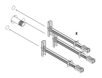
Remove the slide bar from wall and set aside. If there is no stud behind the back plate, utilize the provided high strength toggle anchors (K). Drill a 1/2" hole to push the toggle through. **CAUTION: DO NOT DRILL TOO FAR, WATER LINES AND ELBOW ARE INSIDE THE FINISHED WALL.** Once the toggle is through the wall, slide the cap down the straps until it is flush with the finish wall. Snap off the excess from the straps.
