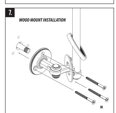
Drill through the tile with 1/8" masonry drill bit. **IMPORTANT:** Stop drilling once you get to the backer board. Apply non-petroleum based lubricant on the 0-rings of the injector. Slide bottom bracket over the injector and ensure the slide bar is level. Use the provided wood screws (M) and mount both dry and wet brackets securely to the finished wall.
