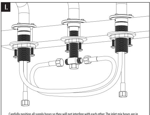
Carefully position all supply hoses so they will not interfere with each other. The inlet mix hoses are in front and do not have the hot or cold label. To avoid kinking, attach the inlet hoses to the opposite side of the T-connection. Connect the inlet mix hoses from the handles as shown. Tighten nut by hand plus 1/4 turn with a wrench until snug. **DO NOT** use teflon tape or plumbers putty.
