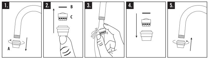
Depending on quality of your household water, the aerator and debris screen may become clogged. We recommend cleaning one week after installation, then a minimum of once of year thereafter. To remove the debris, follow the steps below.
